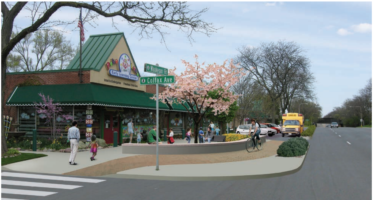
Proposed Improvements: Pick-up and drop-off physically separated from Waukegan. Reverse angle (back-in) diagonal parking increases parking safety and capacity.
