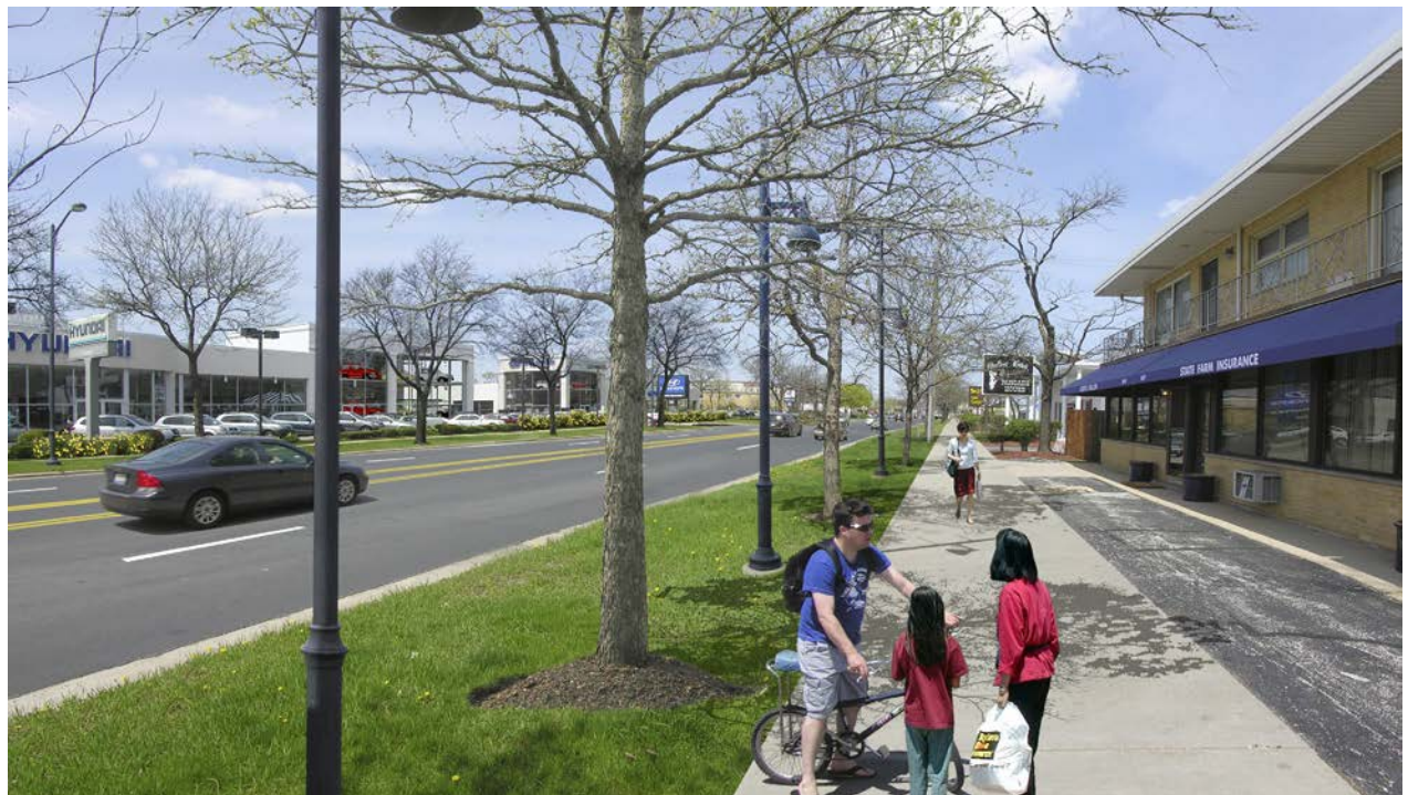
Conceptual Scenarios: 1) Widen existing sidewalk to accommodate 8- to 10-foot multi-purpose path; 2) Alternate tree and street and pathway lighting; 3) Hyundai site improved with multi-story car showroom.
