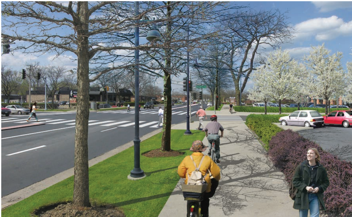
Proposed improvements: 1) Widen existing sidewalk to accommodate 8- to 10-foot multi-purpose path; 2) Remove front portion of Dry Cleaning Factory to accommodate redesigned intersection; 3) Install improved pedestrian crossings; 4) Close multiple curb cuts and reconfigure parking lot; 5) Add low hedge to screen parking area; 6) Extend existing planting strip, add street trees and street and path lighting.
