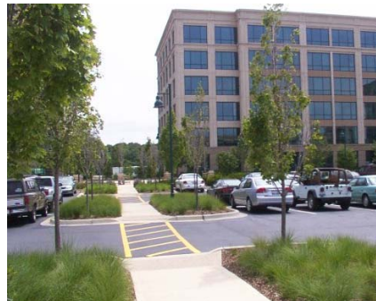
Pedestrian needs are accommodated with a protected walkway through the parking lot
